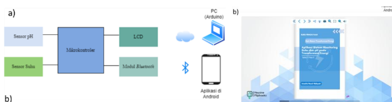
Figure 1. a) Design of pH and Temperature Monitoring System Equipment, b) Enrichment Book Design Development
