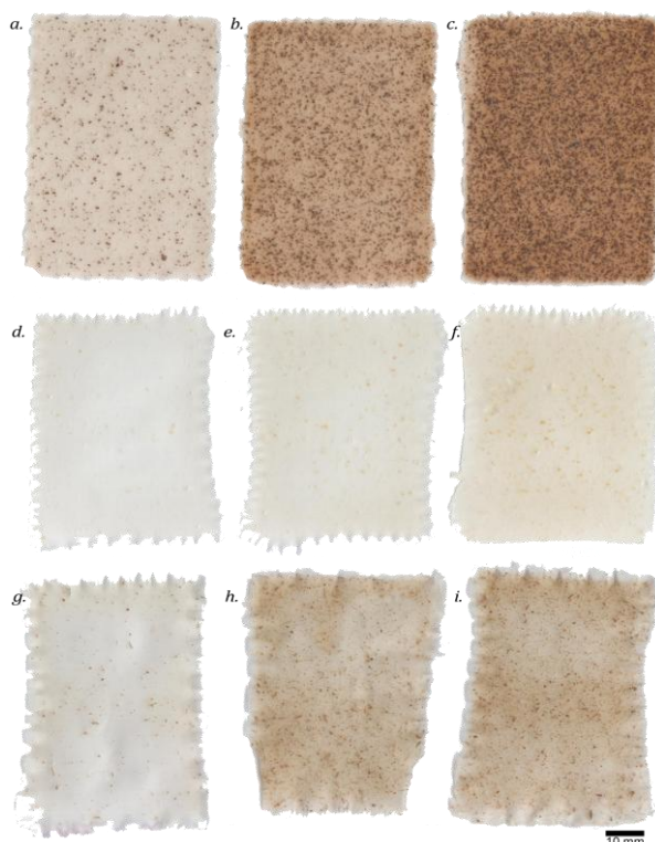
Figure 5. Films with Spent Ground Coffee, Turmeric and Hemp fibres. From right to left: a.) 0.1 % coffee; b.) 0.3 % coffee; c.) 0.5 % coffee; d.) 0.1 % turmeric; e.) 0.3 % turmeric; f.) 0.5 % turmeric; g.) 0.1 % hemp; h.) 0.3 % hemp; i.) 0.5 % hemp.
