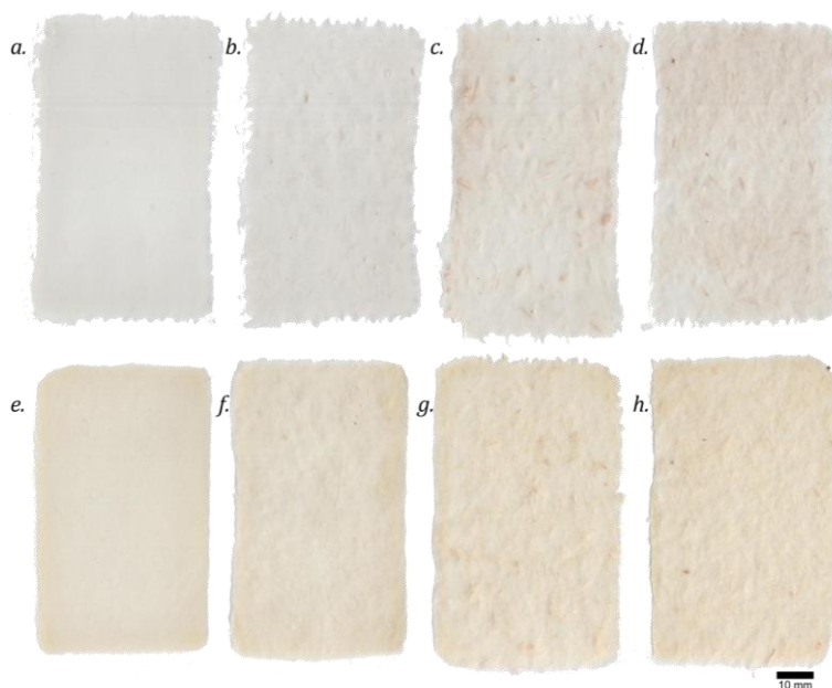
Figure 4. Kenaf fibres-filled films laid on treated wood (a., b., c., and d.) and plastic (e., f., g., h.) a.) and e.) biofilms without filler; b.) and f.) 0.1 % kenaf filler; c.) and g.) 0.3 % kenaf filler; d.) and h.) 0.5 % kenaf filler.
